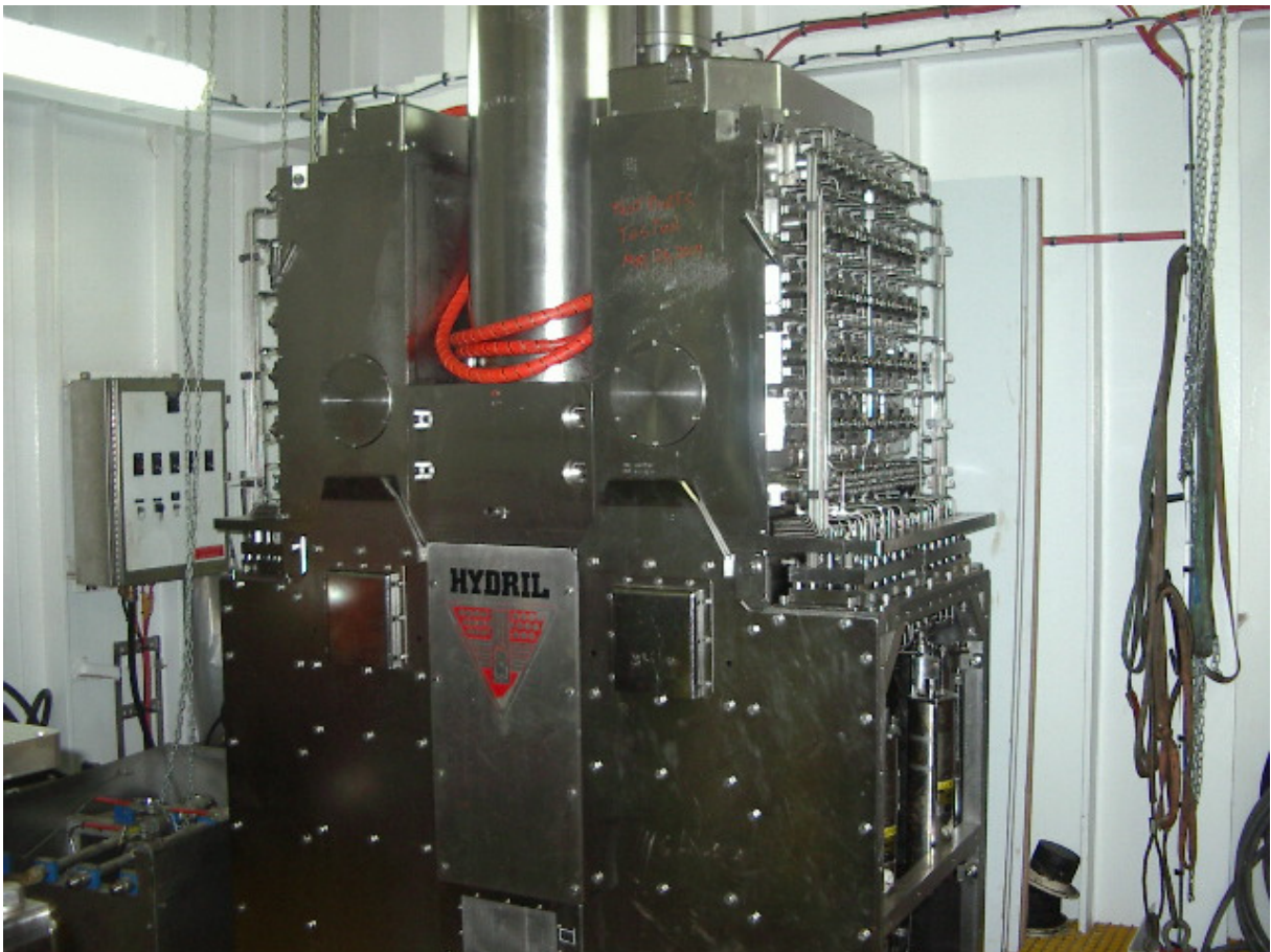
Figura 2.7: POD de controle submarino (GE/HYDRIL, 2013)
