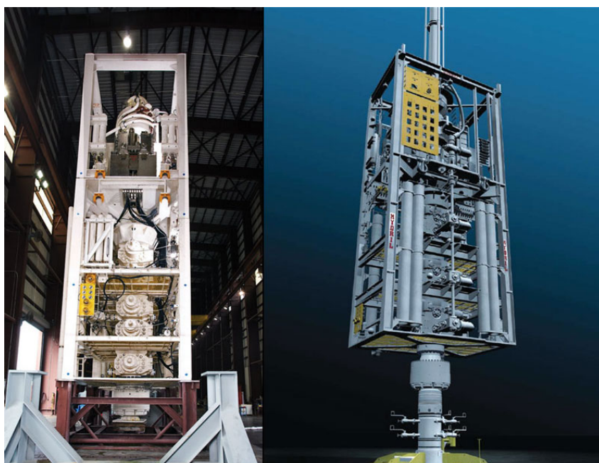
Figura 2.1: Arranjo completo do BOP Stack (GE/HYDRIL, 2013)
